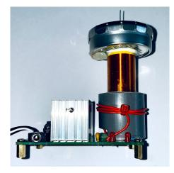
Figure 3: The finished Tesla coil/plasma speaker
